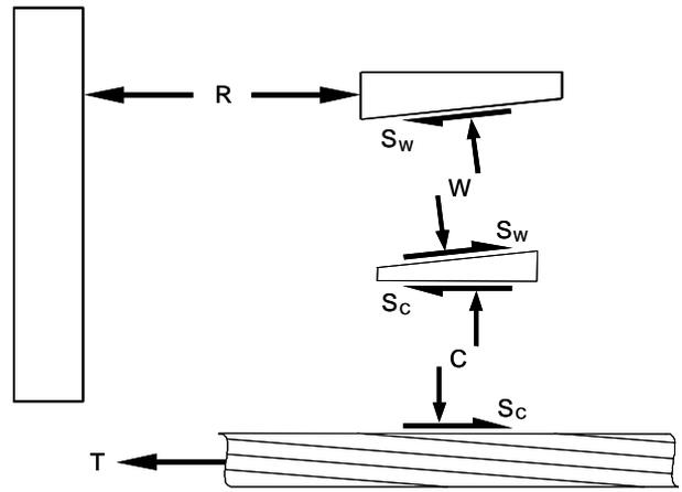
Figure 7: Component forces acting within the strand and barrel and wedge anchor system.
