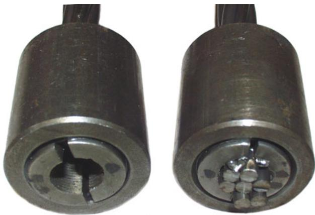
Figure 10: Appearance of anchor specimens 3 and 4 after failure by wedge/strand slip.
