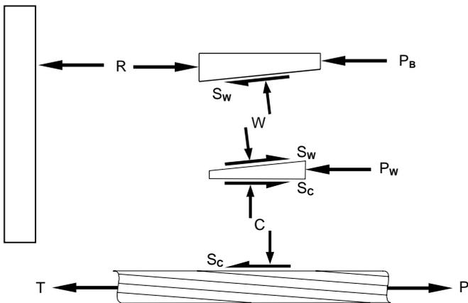
Figure 4: Forces acting on anchor during cable bolt installation.
