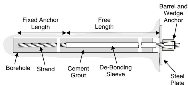
Figure 2: Schematic representation of a cable bolt.
