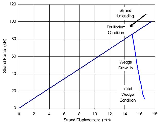
Figure 6: Theoretical prediction of strand tension loss due to wedge draw-in for 5m free strand length initially tensioned to 100kN with 10kN applied to the wedge.
