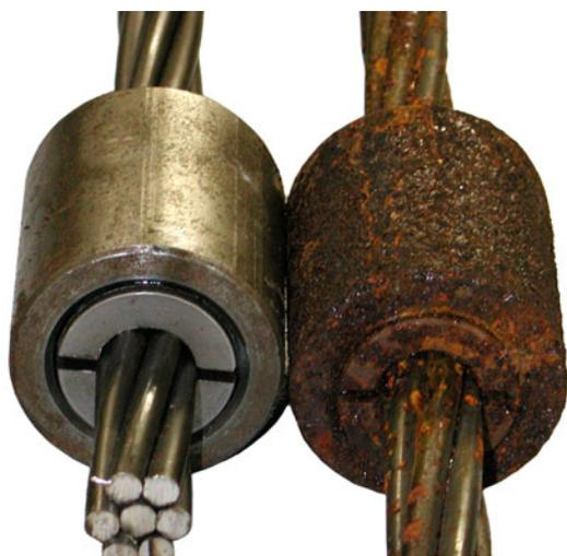
Figure 8: Comparison of new anchor with anchor subjected to 6 months exposure in a mildly corrosive artificial environment.
