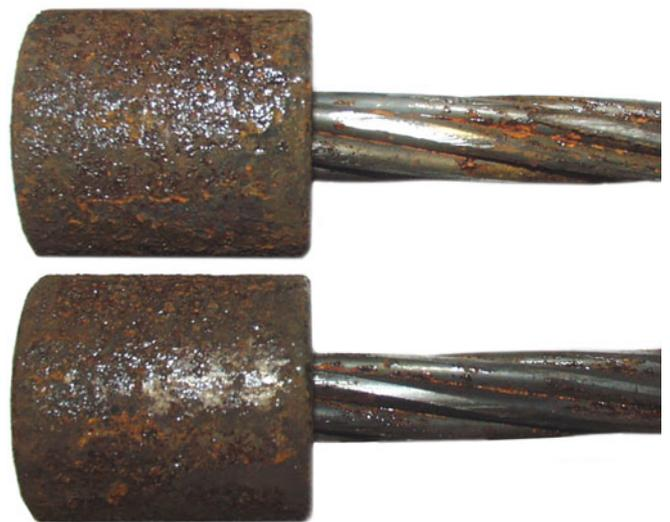
Figure 13: Anchor specimens 6 and 8 after testing (strand slip ~80mm from original position).
