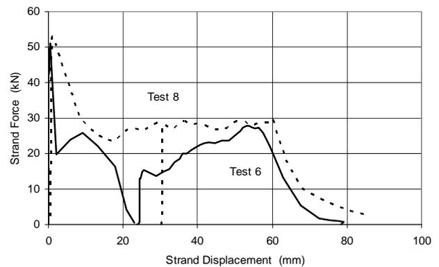
Figure 12: Typical force-strand displacement (Test 6 and Test 8).
