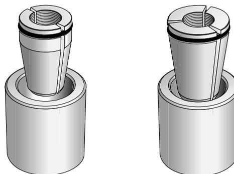
Figure 3: Schematic representation of barrel and wedge anchors with two- and three-part wedges.
