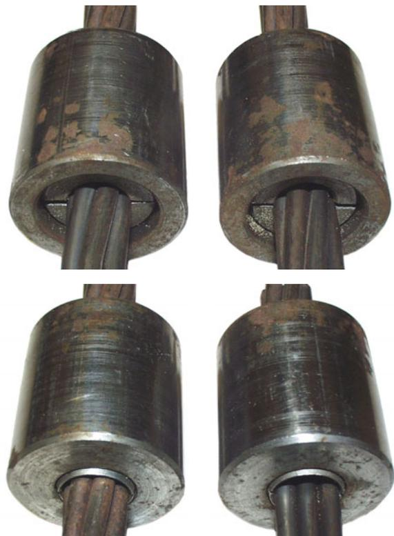
Figure 9: Appearance of new anchors (Specimens 1 & 2) after failure of one and two strand wires.
