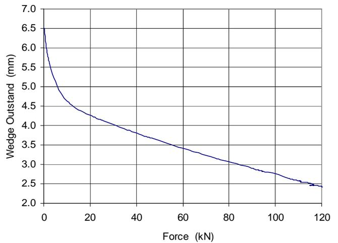
Figure 5: Typical wedge outstand from barrel versus strand force response curve.
