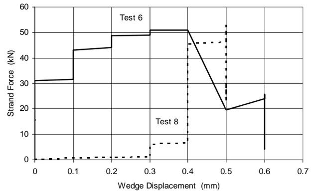
Figure 11: Typical force-wedge displacement (Test 6 and Test 8).
