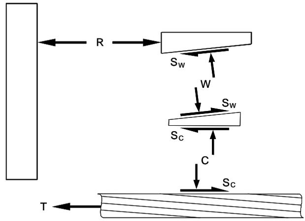
Figure 7: Component forces acting within the strand and barrel and wedge anchor system.
